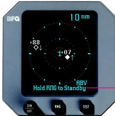
Figure 4-9. Out of Standby on the Ground
