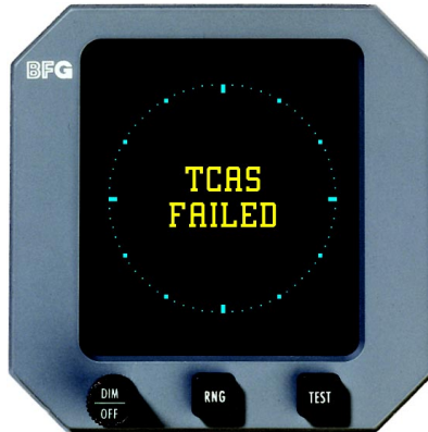
Figure 2-7. TCAS Failed Screen
