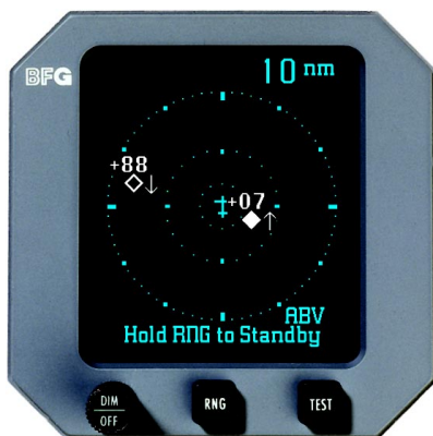
Figure 2-9. Above Display Mode, 10 nmi Range
