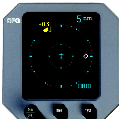
Figure 2-11. Normal Display Mode, 5 nmi Range
