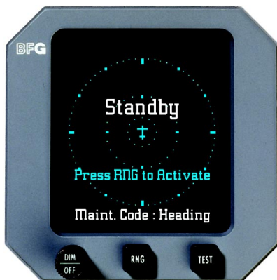
Figure 2-8. Standby Screen with Maintenance Code
