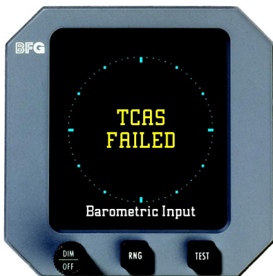
Figure 2-12. TCAS Failed/Barometric Input Screen
