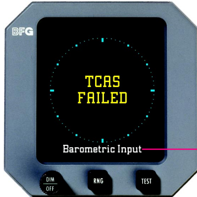
Figure 4-7. TCAS Failed/Barometric Input Screen
