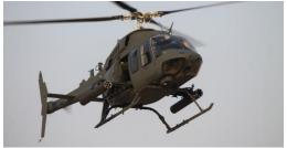
Southeast Aerospace recently delivered the 22nd of 30 heavily modified Bell-407GX aircraft to NorthStar Aviation LLC. After modification, the helicopters, designated as the NSA 407MRH aircraft, are used as a light attack and armed reconnaissance platform by a foreign military customer. Systems include Intelligence Surveillance and Reconnaissance (ISR), Mission Systems and Communications upgrades. The modifications are being completed at SEA's facilities in Melbourne, Florida.
