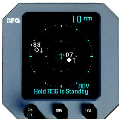
**Figure 2-9. Above Display Mode, 10 nmi Range**
