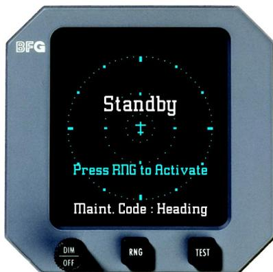
**Figure 2-8. Standby Screen with Maintenance Code**
