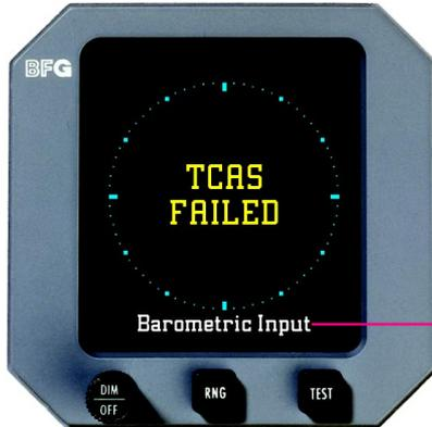
This message indicates that the TCAS791 has failed to detect barometric altitude. If the barometric input is restored, The TCAS791 will return to normal operation.
