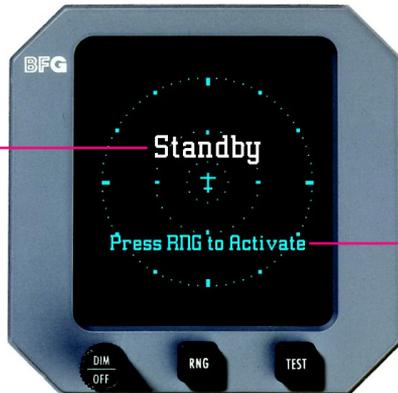
Instructions for switching out of standby and beginning TCAS processing (press the RNG button)
