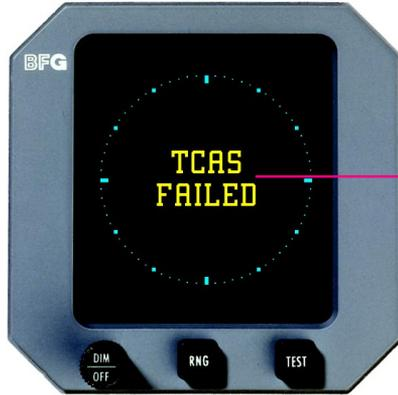
This message is displayed any time the TCAS791 detects a failure. It also appears if the TCAS791 fails the operator-initiated self test. If this message remains on the screen for more than 5 minutes, turn off the TCAS791.
