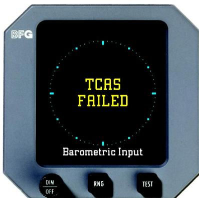
Figure 2-12. TCAS Failed/Barometric Input Screen
