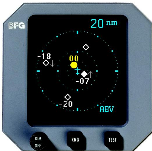
Figure 1-2. Typical Screen on the CD605 Control Display Unit (CDU)
