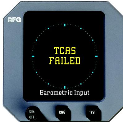
Figure 2-12. TCAS Failed/Barometric Input Screen
