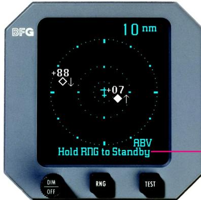
Instructions for switching into standby and stopping TCAS processing (press and hold the RNG button). This message will only appear when your aircraft is on the ground.
