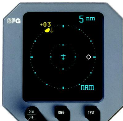
**Figure 2-11. Normal Display Mode, 5 nmi Range**
