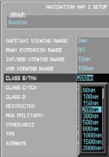
Figure 3-56 Navigation Map Class B/TMA Viewing Range Selection
