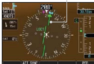
Figure 2-28 Auto-Slewing HSI with ILS Loaded and Shown with the Corresponding Approach Plate
