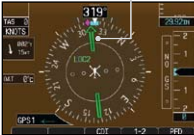
Figure 2-29 Auto-Slewing HSI with Localizer Backcourse Loaded and Shown with the Corresponding Approach Plate
