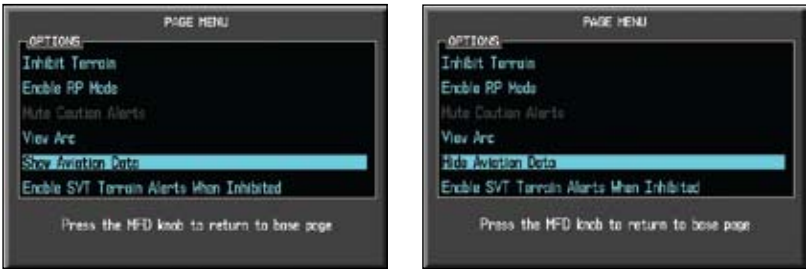
Figure 4-14 Show/Hide Aviation Data on the Terrain-HSVT Page
