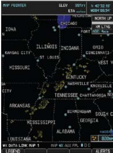
Figure 4-40 XM Weather - Lightning
