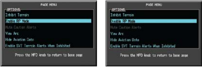
Figure 4-18 Enable or Disable RP Mode on the Terrain-HSVT Page
