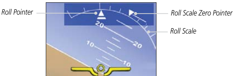
Figure 2-8 Attitude Indicator with a Ground Pointer configuration in a left turn
