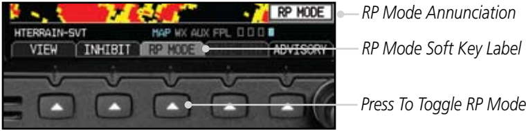
Figure 4-19 Enable or Disable RP Mode on the Terrain-HSVT Page
