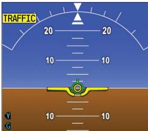
Figure 5-27 Pitch Scale with SVT Disabled
