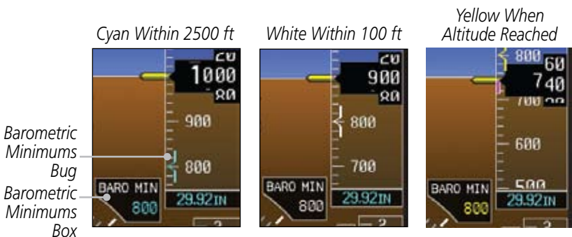
Figure 2-17 Barometric MDA/DH Alerting Visual Annunciations
