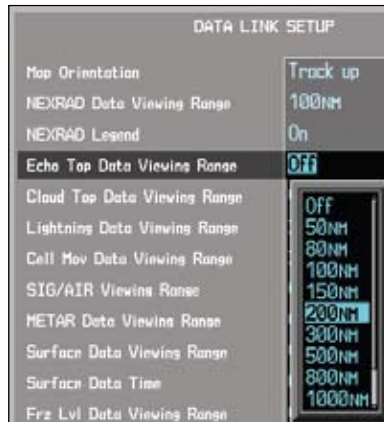
Figure 4-37 Echo Top Viewing Range Selection
