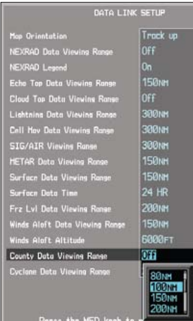
Figure 4-61 County Data Viewing Range Selection
