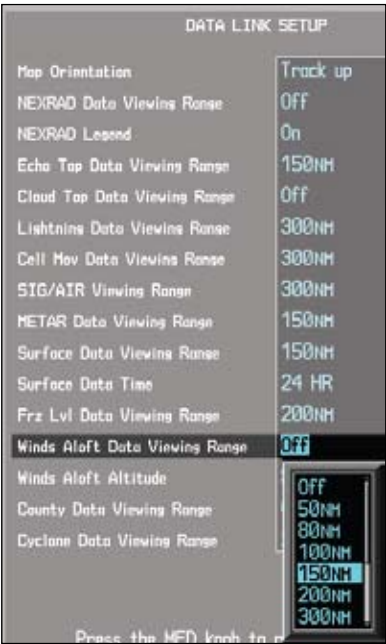
Figure 4-59 Winds Aloft Data Viewing Range Selection
