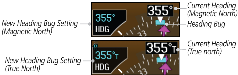
Figure 2-21 Heading Bug Setting
