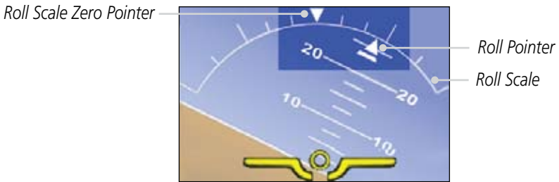
Figure 2-9 Attitude Indicator with a Sky Pointer configuration in a left turn
