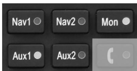
and AUX 2 can be any audio source that is desired at the time of installation, such as ADF, or even an audio alert signal you want to control. The DME input (if present) is also shared with AUX 2.
