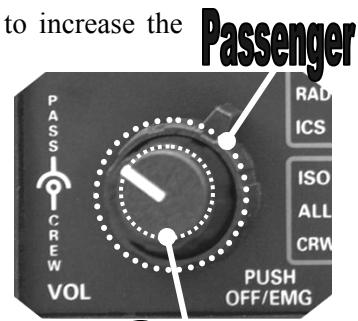
intercom level for the pilot and copilot to the desired level. The volume knob does not affect selected radio levels, music input levels or passengers' intercom volume level.
