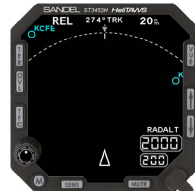
Figure 6-8 Obstacles in REL Display
