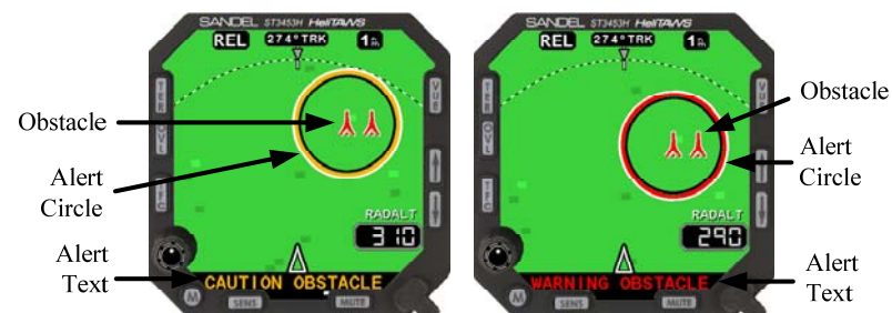
Figure 6-3 Obstacle Alert on a tall tower
