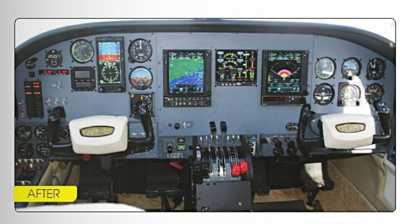
Instrument panels were completely overhauled. An Aspen Evolution 1000 Pro was installed in the pilot's panel. Avionics upgraded to digital J.P. Instruments EDM-960 primary engine data management system, adding a second GTN 750, GWX 70 digital weather radar, GTS 825 traffic system and a Garmin Flight Stream 210. The Avionik Straubing APS4A Altitude Preselect System was installed to complement the S-TEC Autopilot.
