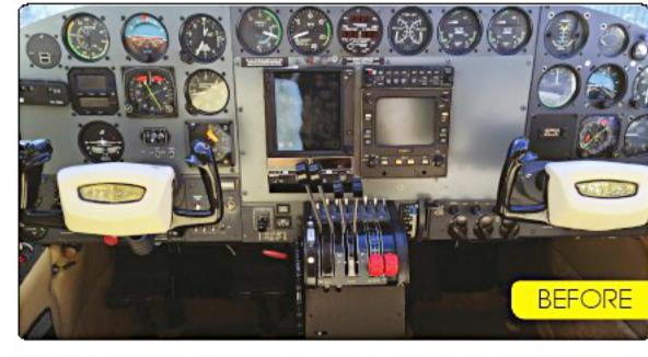
The aircraft arrived with mostly old analog instruments, except for the GTN 750 and a Shadin fuel system. Instrument panel rework had been done at some point.
