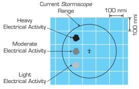
Figure 4-1. Airspace Diagram
