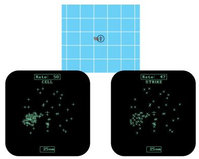
Figure 4-10. Cluster and Splattering Within 25 nmi
