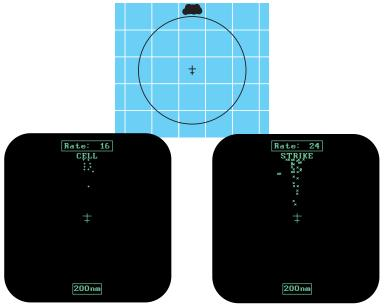
Figure 4-11. Discharge Points Off Aircraft's Nose
