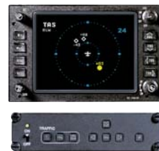
Radar Indicator via the RGC350
