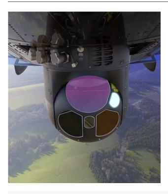
The Star SAFIRE® 380X-HD provides enhanced features in a single LRU for defense, airborne law enforcement, SAR units, and airborne firefighting applications. Advanced image aiding features reduce operator workload for faster, smarter decision support and features customizable configurations and icon-based graphics, multi-tile video management and external video input from another system.
