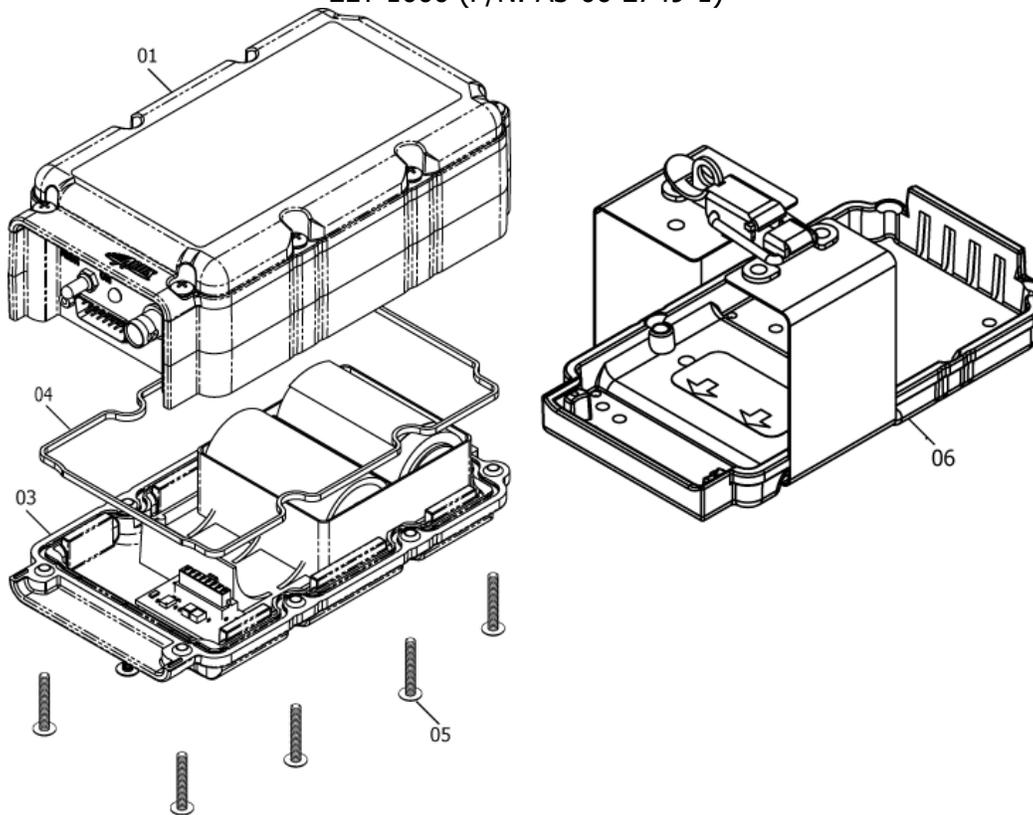
**Figure 29 ELT 1000 Main Assembly and Installation**
