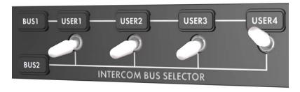
If one user is to be **ISOLATED** from the other users, that user must be connected to a different bus to all the other users. (i.e. User's switch must be in the opposite direction to all the others.) In this example, User 4 is isolated from Users 1, 2 and 3.
