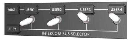
If it is necessary to **SPLIT** the users into Talk Groups, (for instance Flight Crew and Cabin Crew) the users' switches should be connected to different busses (in this example, User 1 and User 2 are connected on BUS 2; User 3 and User 4 are connected on BUS 1.
