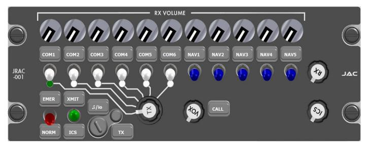
From the Virtual Control Panel it is possible to adjust the switches 'on' and 'off' by clicking on them, and to adjust the rotary controls by 'dragging' them round.
