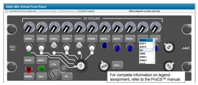
This Virtual Front Panel is used to define the 'names' associated with the control legends. The selected name will be used in all subsequent references to the associated transceiver/receiver, and will be used on the custom-generated Connector Maps and Interconnects. Also see section 2.6 (Virtual Control Panel).
