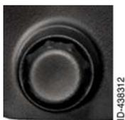
Rotating the outer knob of the radio control knob tunes the selected radio standby megahertz (MHz) frequency (the digits to the left of the decimal point). Rotating the inner knob tunes the selected radio standby kilohertz (kHz) frequency (the digits to the right of the decimal point). Pushing the knob toggles the COM and NAV frequencies.
