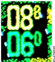
**EGPWS Peaks Elevation** - The numerical maximum peaks elevation is displayed above the numerical minimum peaks elevation. Peaks elevation is displayed for all installations.
