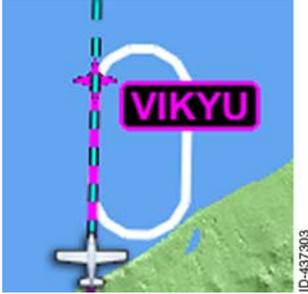
**Holding Patterns** – Holding patterns are represented by a symmetrical oval racetrack symbol. Holding pattern entries are displayed when the FMS recommends a teardrop or parallel hold entry.
