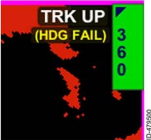
The terrain view uses the magnetic heading from the magnetic ground track of the internal global positioning system (GPS) if the heading of the aircraft is invalid or unavailable and TRK UP (HDG FAIL) is displayed in the upper-right corner of the terrain view.
