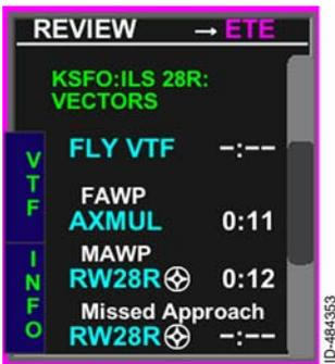
**Vectors to Final** – The vectors to final selection provides a final approach extension from the FAWP that can be used to orient the flight crew while being vectored to the final approach. Vectors to final leg is indicated in the flight plan list as **FLY VTF**.
