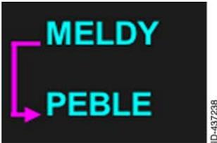
**Current Segment** – When autopilot GPSS is available, the current segment of the flight plan is indicated with a magenta arrow, which shows the From waypoint and the TO waypoint. Also, the TO waypoint and active leg are displayed in magenta on the map display.
