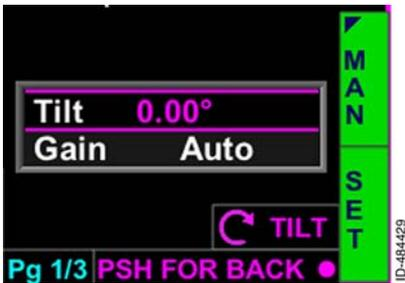
Manual tilt is selected by activating the **MAN** bezel softkey label. The default tilt value is the last commanded manual tilt value and is displayed in the manual tilt field. Manual tilt mode has a range of  $\pm 15.0^\circ$ .  $-15.0^\circ$  represents the extreme counterclockwise rotation and  $+15.0^\circ$  represents the
