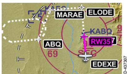
**Missed Approach Procedures** – The missed approach procedure is displayed as white dashes until the missed approach is activated. When activated, the missed approach procedure is displayed as normal flight plan legs.
