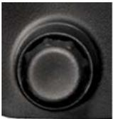
Rotating the outer knob of the **radio control knob** tunes the selected radio standby megahertz (MHz) frequency (the digits to the left of the decimal point). Rotating the inner knob tunes the selected radio standby kilohertz (kHz) frequency (the digits to the right of the decimal point).
