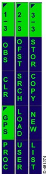
When the FMS window has focus, three pages of bezel softkey labels can be alternated for display along on the right-side of the display. These bezel softkey labels allow the pilot to operate various FMS functions.
