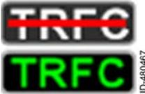
When a TAS TCAS sensor is installed and traffic information is in a failure status, the TRFC annunciation is displayed in white text with a red line through. When a TAS TCAS sensor is installed and valid traffic information is being received, the **TRFC** annunciation is displayed. When a TIS TCAS sensor is installed and traffic information is unavailable or out of range, the **TRFC UNAV** annunciation is displayed.
