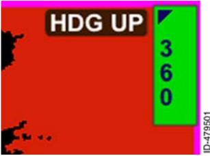
When in the terrain view and the heading is available, HDG UP is displayed in the upper-right corner of the terrain view.
