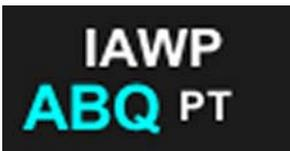
**Procedure Turn Indication** – When a waypoint requires a procedure turn, **PT** is displayed after the name of the waypoint.
