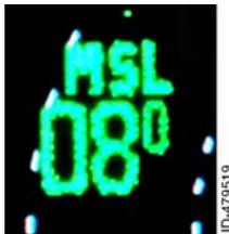
**EGPWS Mean Sea Level (MSL) Altitude** - The displayed MSL altitude is the computed Geometric altitude which is the internal calculation of the current MSL altitude. The EGPWS MSL altitude is only displayed for KGP 560/860 and KMH 880/980 installations.
