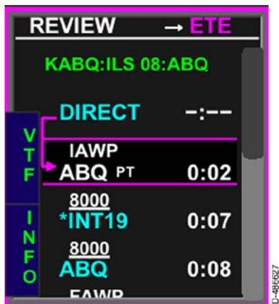
Procedure turns are associated with approach procedures. The turns are used for course reversals to align the aircraft with the runway. When an approach procedure contains a procedure turn, the FMS displays the procedure turn as a canted teardrop symbol on the navigation map display and displays **PT** next to the procedure turn waypoint in the waypoint list.
