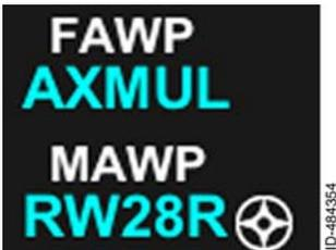
**Initial Approach, Final Approach, and Missed Approach Waypoints** – **IAWP**, **FAWP**, and **MAWP** headings are displayed above the initial approach waypoint, final approach waypoint, and missed approach waypoint, respectively, when an approach procedure is loaded into the flight plan.
