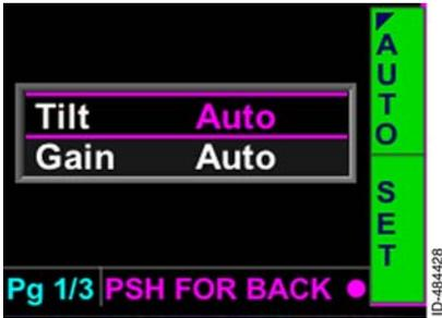
Auto tilt mode is selected when the **AUTO** bezel softkey label is active. The tilt annunciation field displays **Tilt Auto**. Auto tilt permits the antenna position to be automatically adjusted to maintain a common beam intercept point with the earth. For example, if the last 10% of the display is ground
