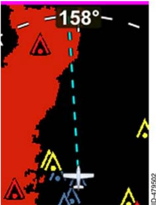
In heading-up or track-up mode, the direction of flight value displays the heading/track with a resolution of 1 degree and a range of 1 to 360 degrees.
