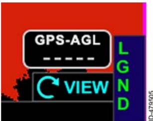
The AGL value is dashed ( **-----** ) when there is no terrain coverage for the present position, or when the AGL value is above 51,000 feet or below 500 feet.
