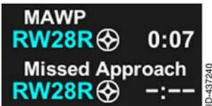
**Missed Approach** – The **Missed Approach** header in the waypoint list window is used to separate the flight plan from the missed approach procedure.
