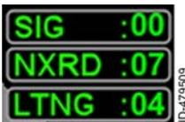
The XM product ages box is displayed in the lower-left corner of the navigation map and datalink weather pages. The XM product ages for the selected weather products are displayed (in minutes) in green when data is being received and updated.
