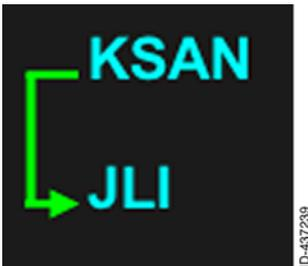
When autopilot GPSS is not available, the current segment of the flight plan is indicated with a green arrow that shows the From waypoint and the To waypoint. Also, the TO waypoint and active leg are displayed in green on the map display.
