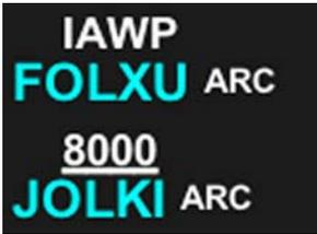
**Arc Turn Indication** – When a waypoint defines the beginning or end of an arc turn (for example, a DME arc or a radial to a fix), **ARC** is displayed after the name of the waypoints that define the beginning and end of the arc turn.
