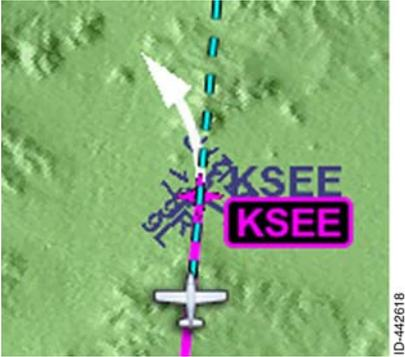
**Guidance Arrow** - When the active flight plan has two consecutive legs and the desired track of the second leg has a large change, a white arrow is displayed from the first leg to provide pilot-awareness to the direction the FMS is providing guidance.
