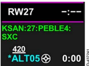
**Flight Plan Procedure Banner** – Loaded procedures in the flight plan are displayed in green text prior to the first waypoint of the procedure in the flight plan list.
