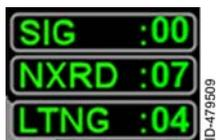
The XM product ages box is displayed in the lower-left corner of the navigation map and datalink weather pages. The XM product ages for the selected weather products are displayed (in minutes) in green when data is being received and updated.
