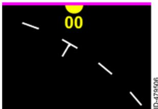
TAs outside the current range are indicated by a half-symbol at the edge of the display with the correct data block. Proximity advisories and other traffic outside of the current range are not displayed.
