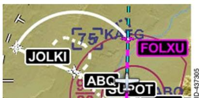
**Arc Turns** – Arc turns are represented by a curved line between the two waypoints that define the beginning and the end of the arc turn.
