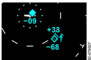
When multiple traffic symbols partially or completely overlap, the symbols are visually stacked, with the highest priority alert data on top, obscuring the lower priority alert. When a traffic symbol and the ownship symbol partially or completely overlap, the traffic symbol and data block will overlay the ownship symbol and indicate if the traffic is above or below the aircraft.
