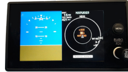
Multifunction Displays Integrated multipurpose display supporting primary flight information
