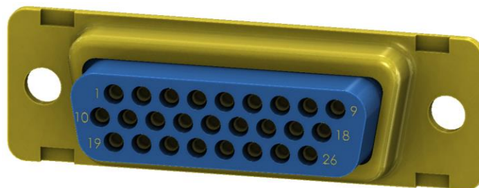
Figure 3.1 View from Rear of Mating Connector
