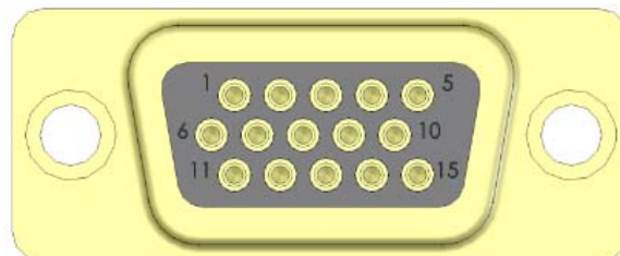
FIGURE 3.1 VIEW FROM REAR OF MATING CONNECTOR
