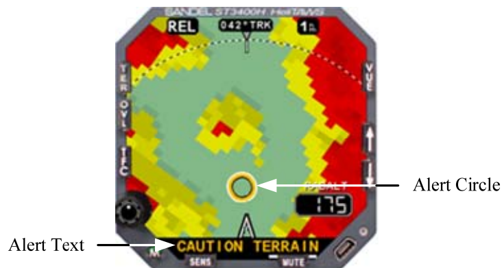
Figure 6-1 “CAUTION TERRAIN” Annunciation
