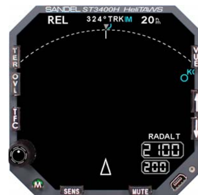
Figure 6-8 Obstacles in REL Display
