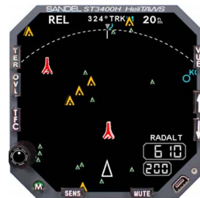
Figure 6-7 Obstacles in REL Display
