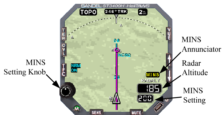
Figure 8-1 Radar Altimeter Functions
