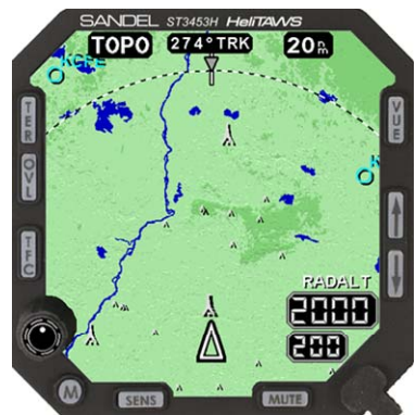
Figure 6-6 Minimized Obstacles in TOPO Display
