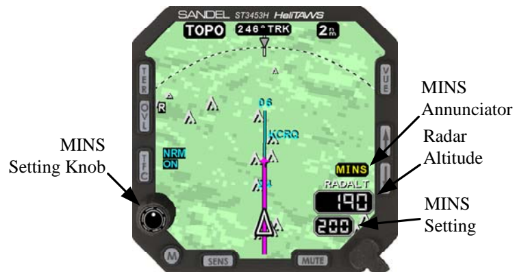
Figure 8-1 Radar Altimeter Functions
