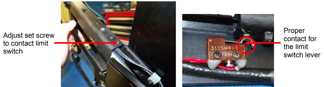
Figure 15 Set screw and limit switch positions for power on/off control
